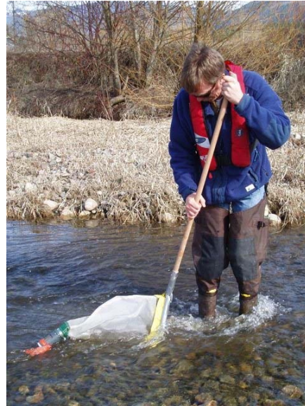
Using a kick net to sample benthic invertebrates. Photo credit: Carolyn Johns
