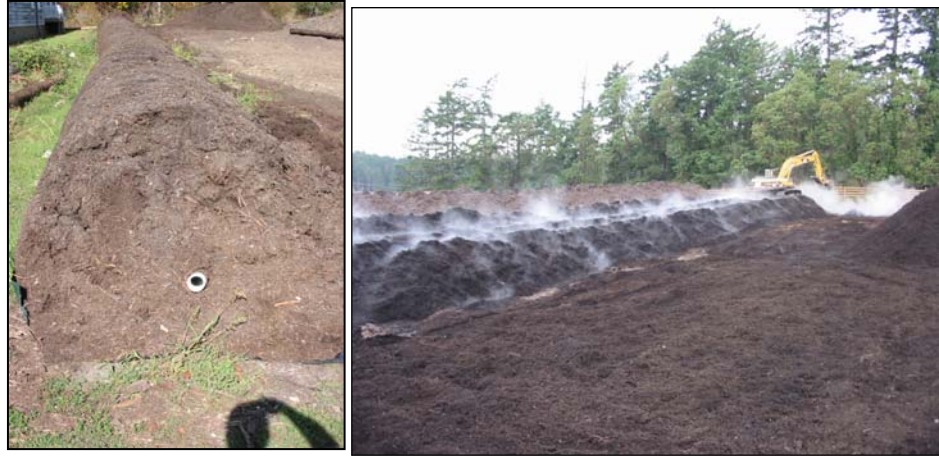
Figure 1 On the left is a variation of the aerated static pile using an Ag-Bag (bag removed). Note the perforated pipe used to pump air through the pile to maintain aerobic conditions during composting. On the right, the photo shows open windrows of compost with steam rising from the windrows.
