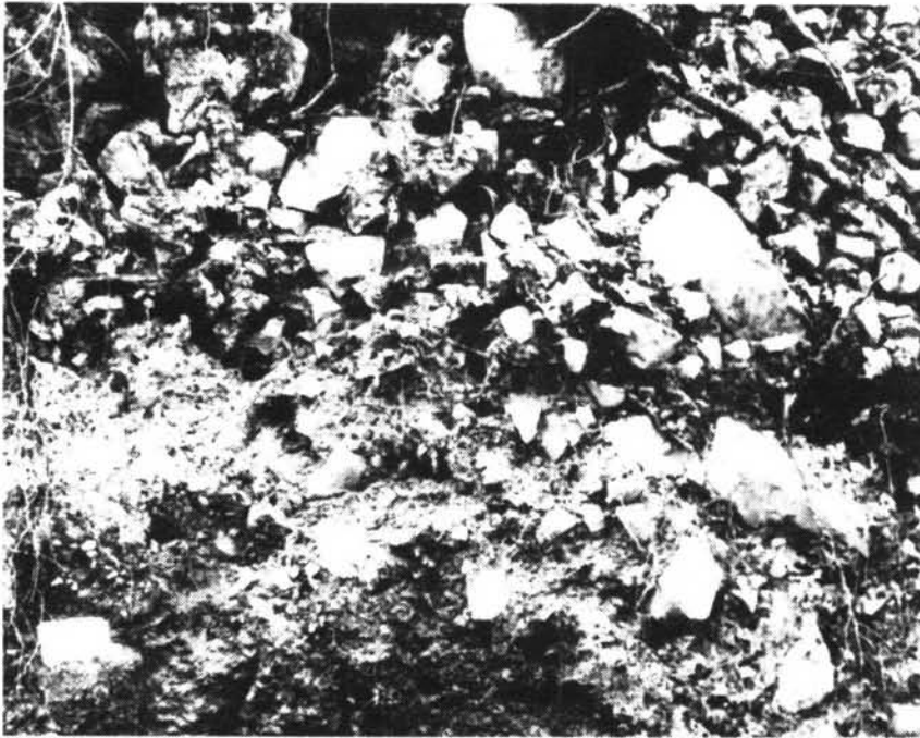
Plate 7. Deep colluvial deposit (greater than 5 feet deep) derived from shattered bedrock.
