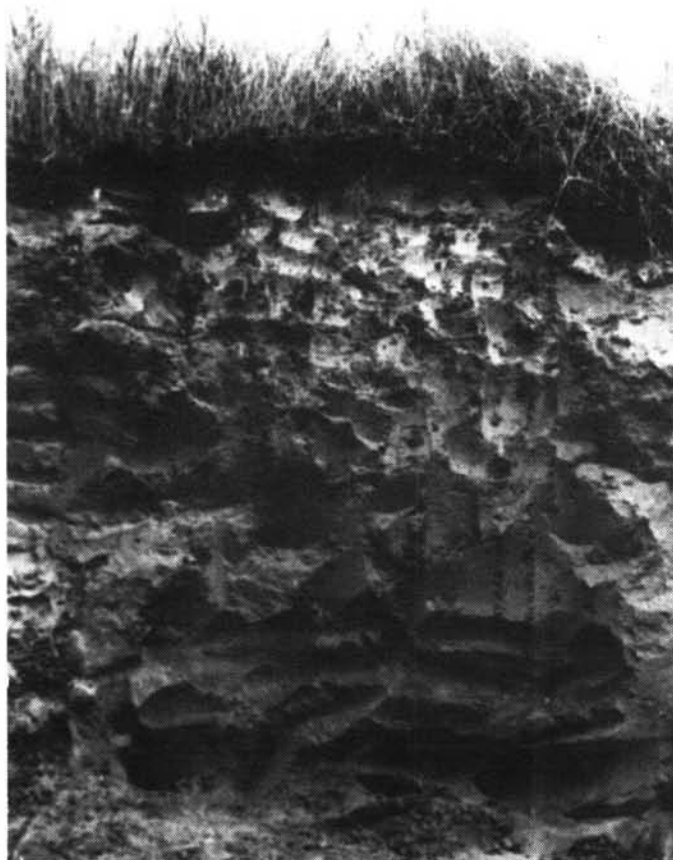
Plate 13. Sandy loam alluvial parent material with Degraded Eutric Brunisol soil development. The Ae horizon near the surface is easily discerned.
