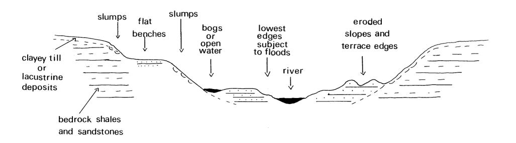
Figure 1 Generalized Cross Section of the valley
