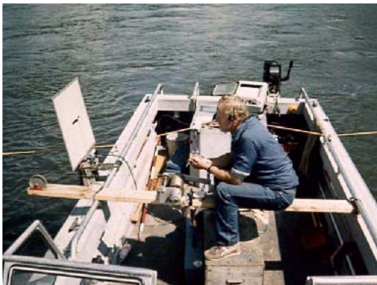
Figure 57: A55 reel and bridge board mounted in boat (Nechako River).
