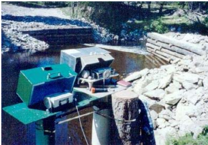
Figure 70: Two water level recorders: a data logger and an analogue recorder.
