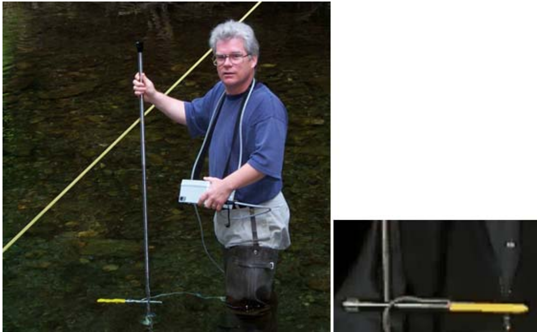
Figure 41: OTT Nautilus C 2000 Electromagnetic Flow Sensor (0 – 2.5m/s).
