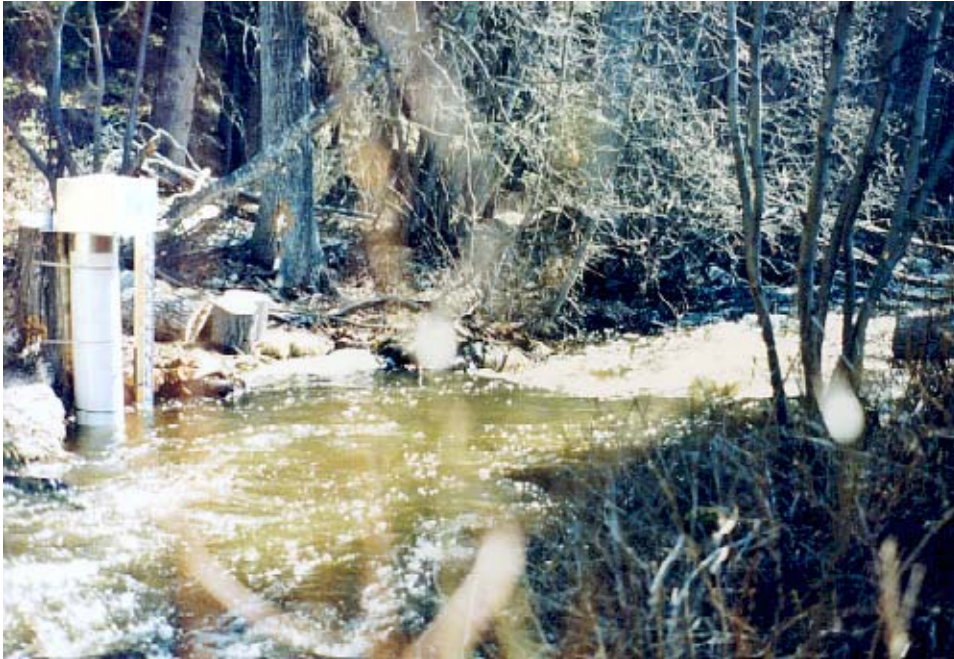
Figure 72: Boulder control (subject to debris build-up) and water level recorder stilling well and shelter. Narcosli Creek, above Ramsay Creek, West Fraser.
