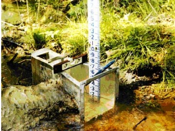
Figure 73: Three-inch Portable Montana flume set in a temporary mud dam.
