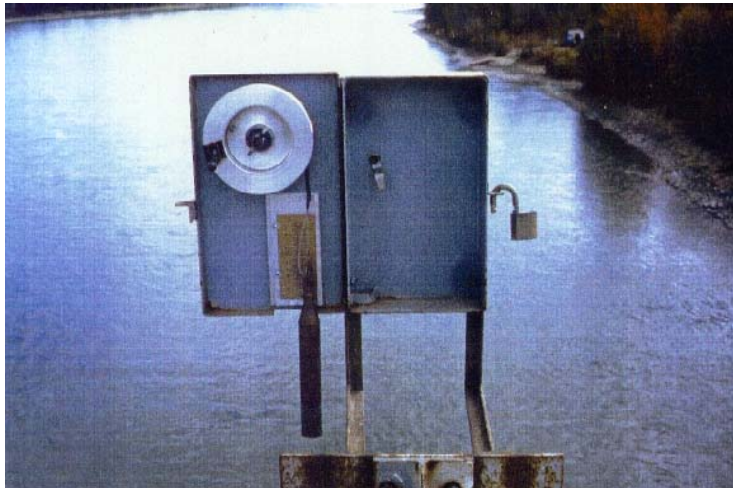
Figure 26: Wire-weight gauge and mounting brackets. Athabasca River, near Windfall (Courtesy: WSC).
