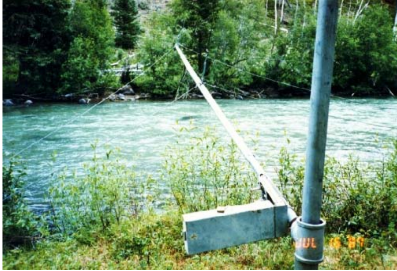
Figure 25: Boom wire weight gauge.
