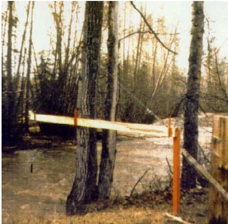
Figure 24: Chain gauge (Courtesy: WSC).
