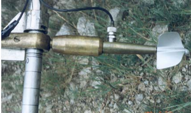
Figure 40: OTT C2 Current Meter (Horizontal Axis Meter) .
