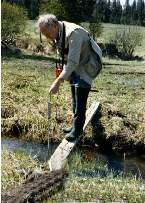
Figure 50: Ditch flow measurement using planks.
