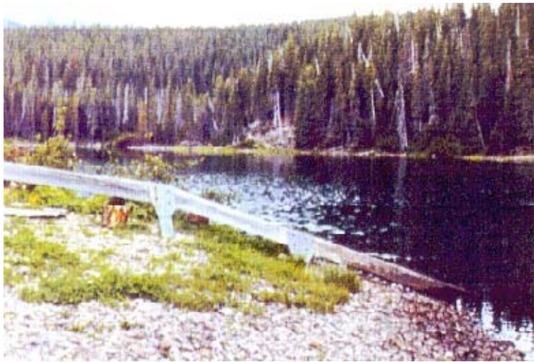
Figure 27: Inclined gauge with metal tags between the metre markers (Courtesy: WSC).
