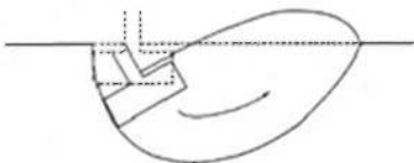
Figure C1-a: Local Bearing Failure
