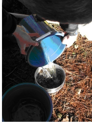
Figure 19 – Elutriation using several buckets
