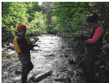
Figure 15 – Example of field crew collecting water quality information with a multi-probe (wearing appropriate personal protective equipment)
