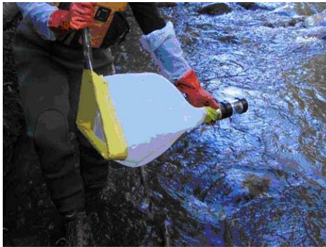
Figure 17 - Triangular kick net with 400 \mu\text{m} mesh net and detachable collection cup
