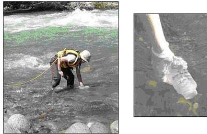
Figure 14 - Safe and proper water sampling technique
