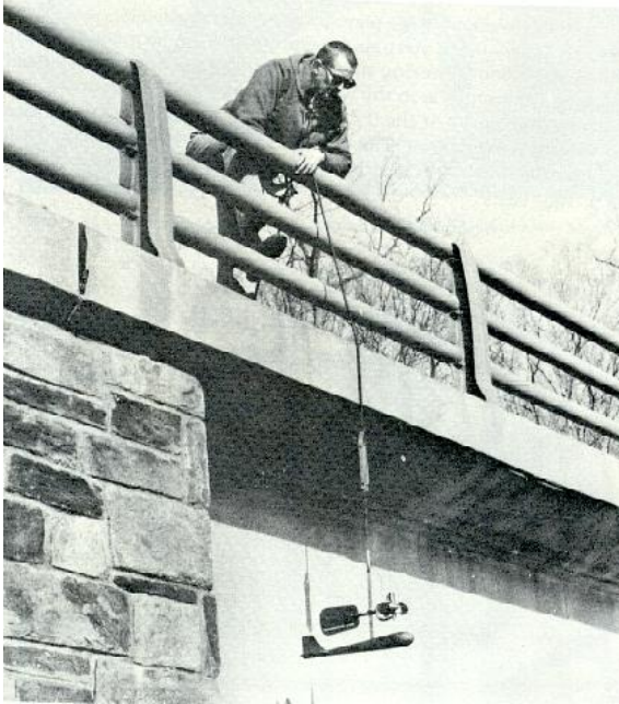
Figure 56: Handline in operation (Source: USGS Water Supply Paper 2175 Vol. 1).
