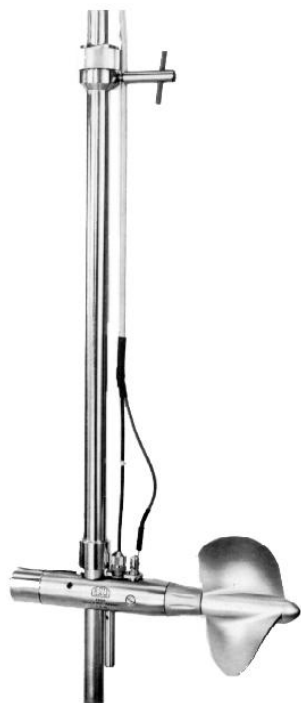
Figure II-7. OTT C31 current meter fitted on a 20-mm rod, with relocating device. Note that the locating device, at top, is aligned with a meter.
