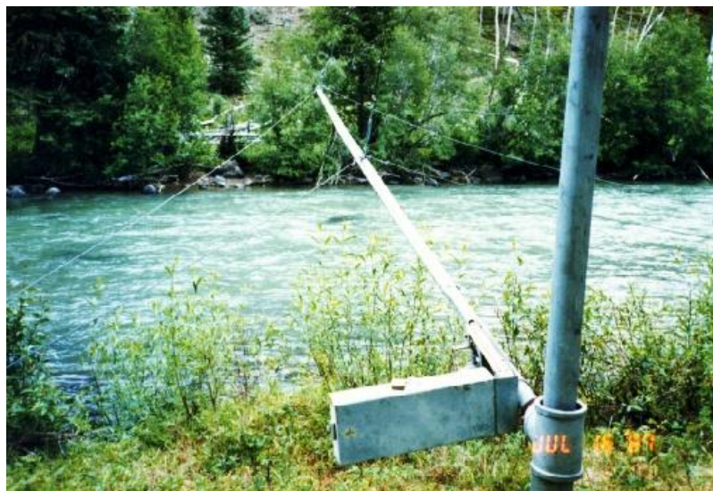
Figure 25: Boom wire weight gauge.
