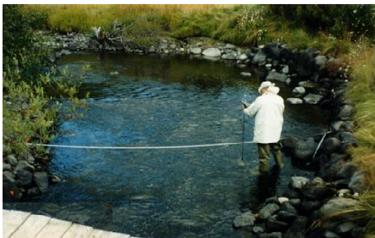
Figure 51: Conducting a discharge measurement with tagline across the wading section, Bridge Creek below Deka Creek.
