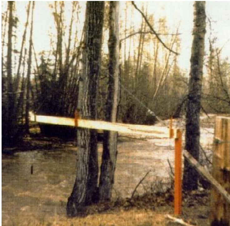
Figure 24: Chain gauge (Courtesy: WSC).
