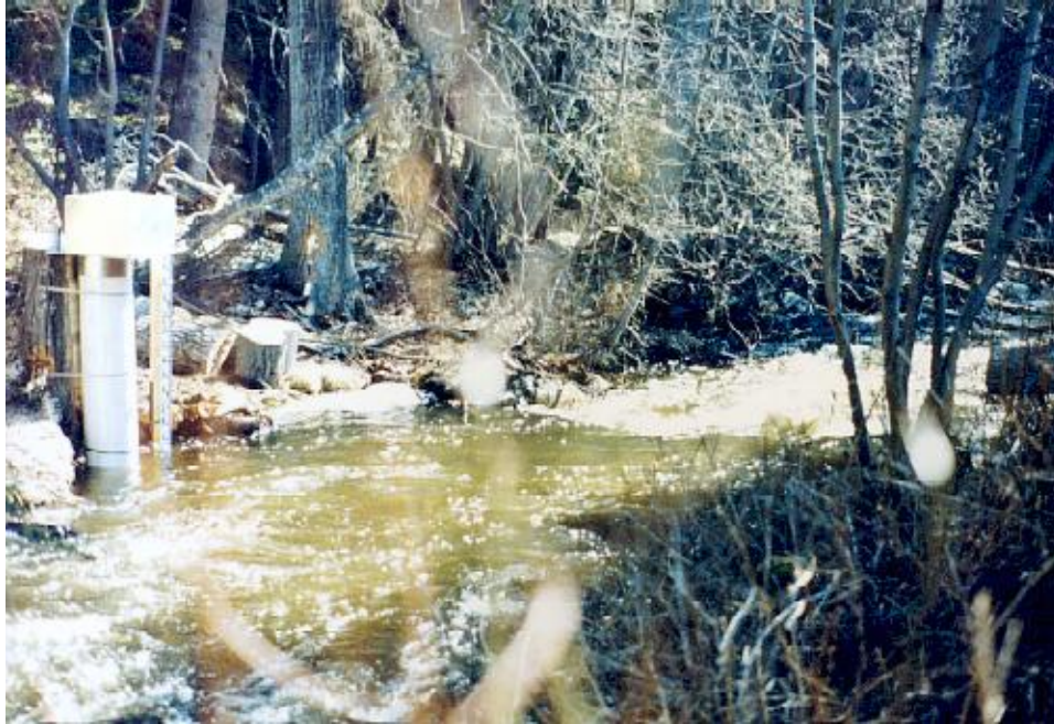
Figure 72: Boulder control (subject to debris build-up) and water level recorder stilling well and shelter. Narcosli Creek, above Ramsay Creek, West Fraser.
