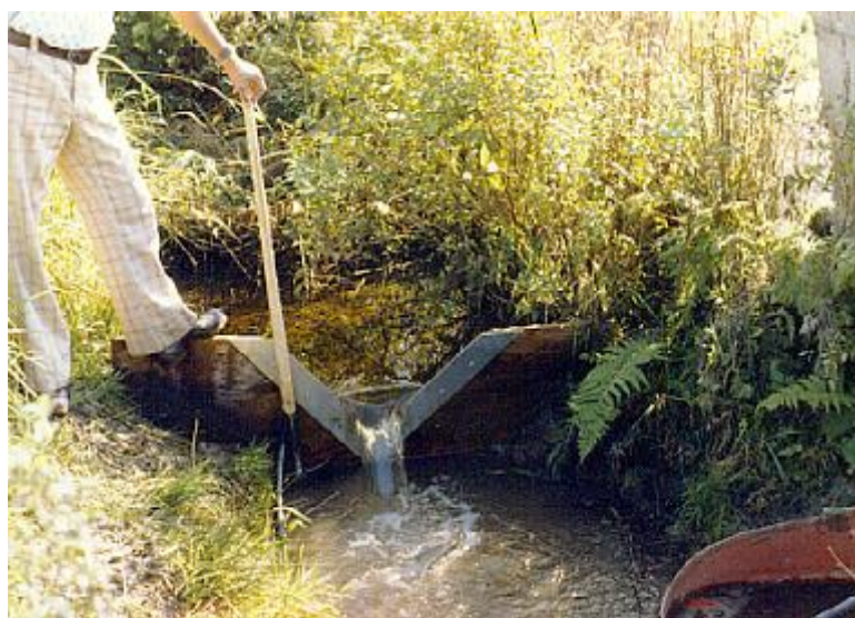
Figure 74: V-notch weir plate, portable installation.
