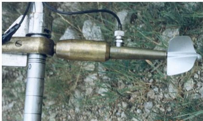
Figure 40: OTT C2 Current Meter (Horizontal Axis Meter) .
