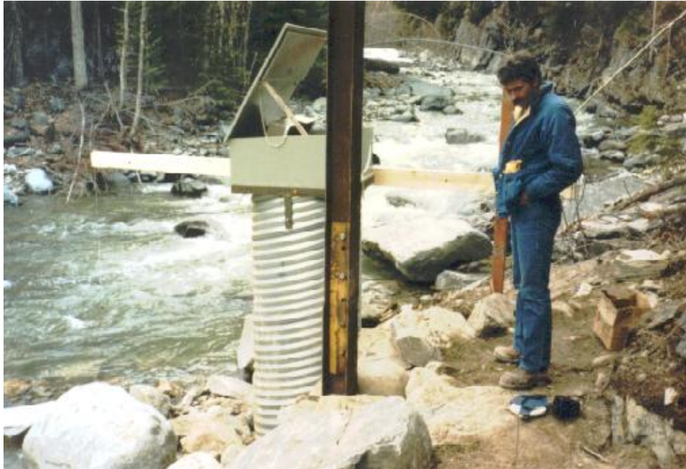
Figure 34: In-bank stilling well.
