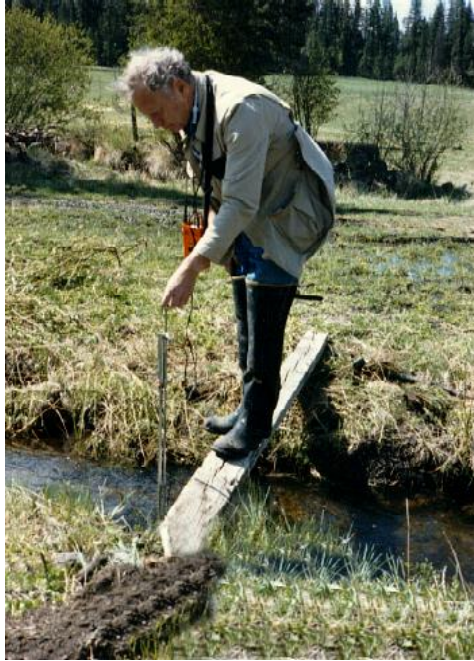
Figure 50: Ditch flow measurement using planks.
