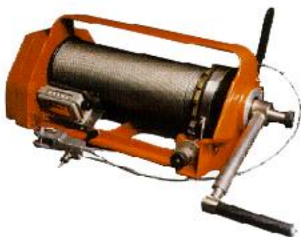
Figure 46: San sounding reel, made in Australia.
