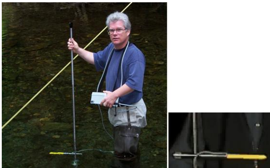
Figure 41: OTT Nautilus C 2000 Electromagnetic Flow Sensor (0 – 2.5m/s).
