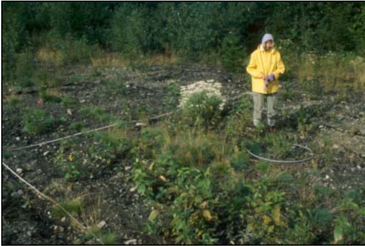
Figure 14. Sampling the density and cover of native plants sown on an old log sort yard.
