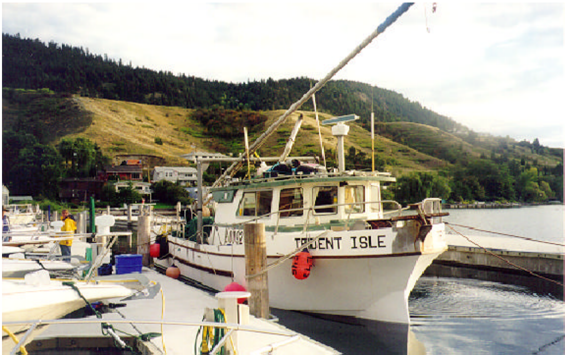
Photo 2. 13 m Trident Isle commercial fish boat with 16.5 m aluminum beam stored atop of wheelhouse and net drum (aft).
