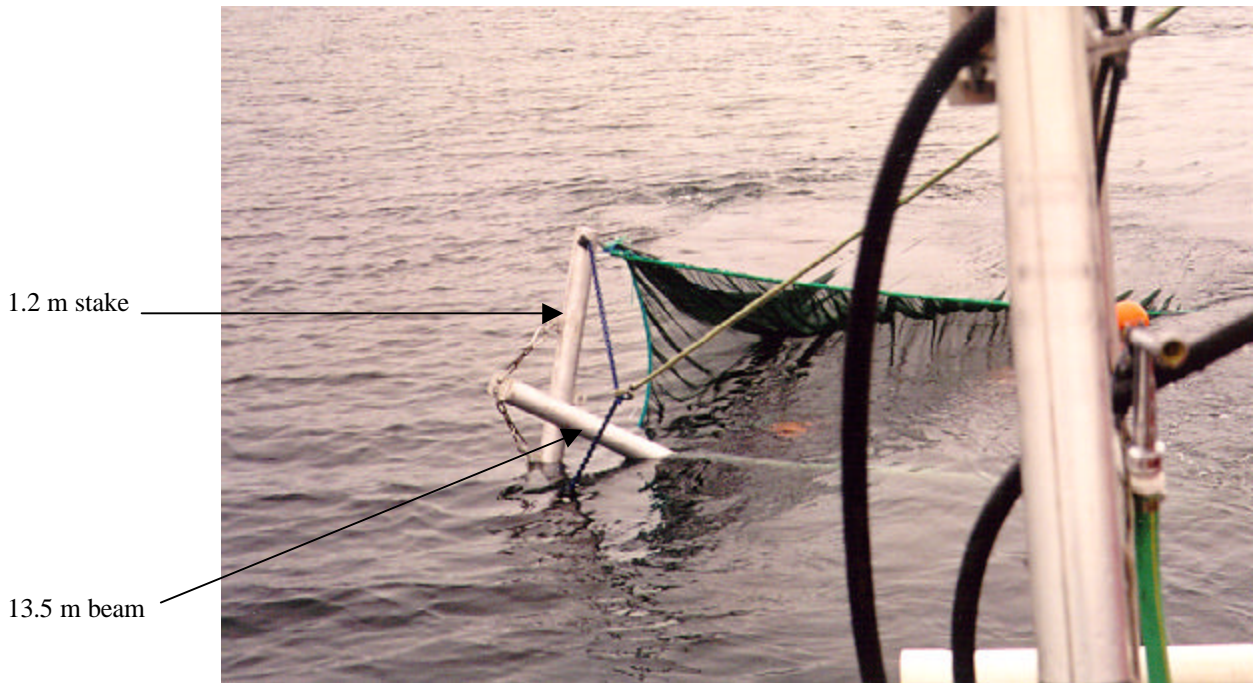
Photo 1. Deployment of 1998 prototype net illustrating 1.2 m stake, 13.5 m beam and bridle attached to single cable mounted on the boats net drum.
