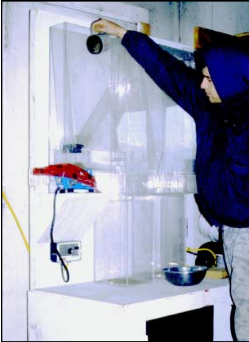
Figure 10. A vacuum aspirator used for final separation of filled seeds from dust, chaff, and unfilled seed, based on differential buoyancy in an air stream.
