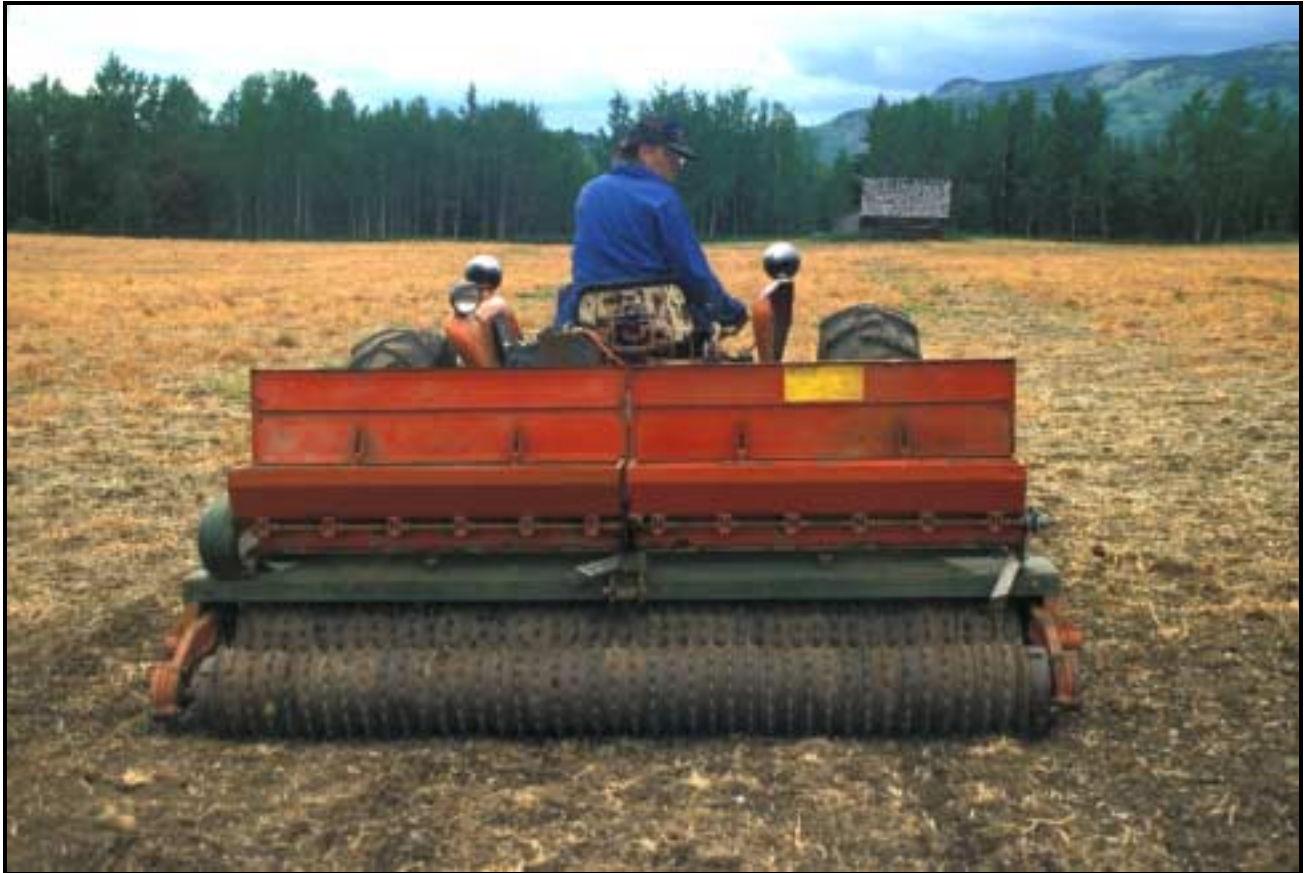
Figure 3. Spring-sowing a native grass using a small (Brillion™) seed drill pulled by a tractor for establishment of a small seed production field. Row spacing here is approximately 12 cm.
