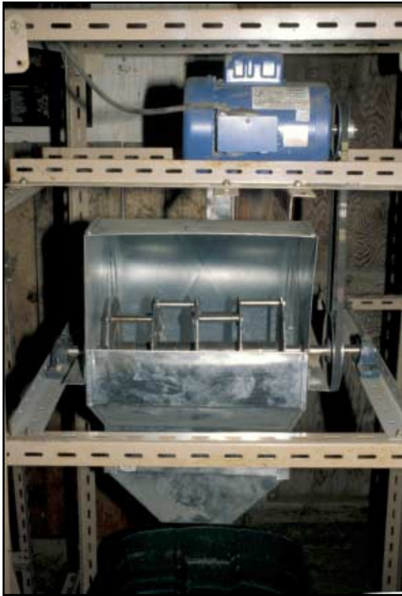
Figure 8. Custom-made rotary flail, mounted with housing and electric motor. Heads of long seed stalks are held into the unit, with the seeds knocked out of seed heads by the rotating bolts mounted horizontally between the vertical discs.
