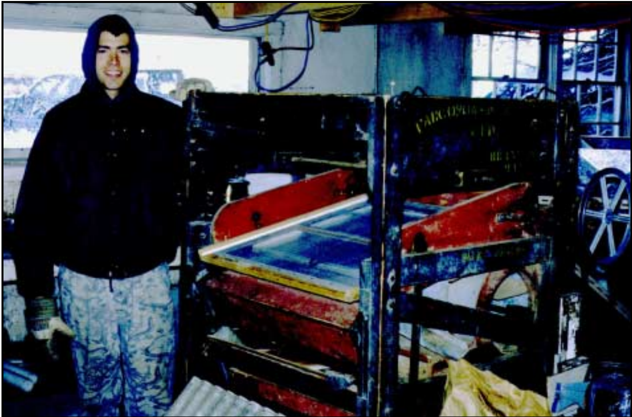
Figure 9. A small fanning mill or “air-sieve machine” used for seed cleaning.
