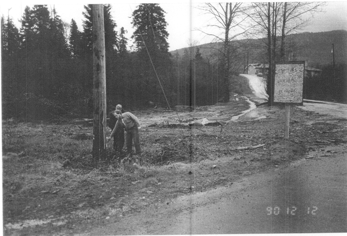
Photo 18 High water mark (nail in power pole) from December 4, 1990 flooding. This is on the left bank just downstream of XS-26.
