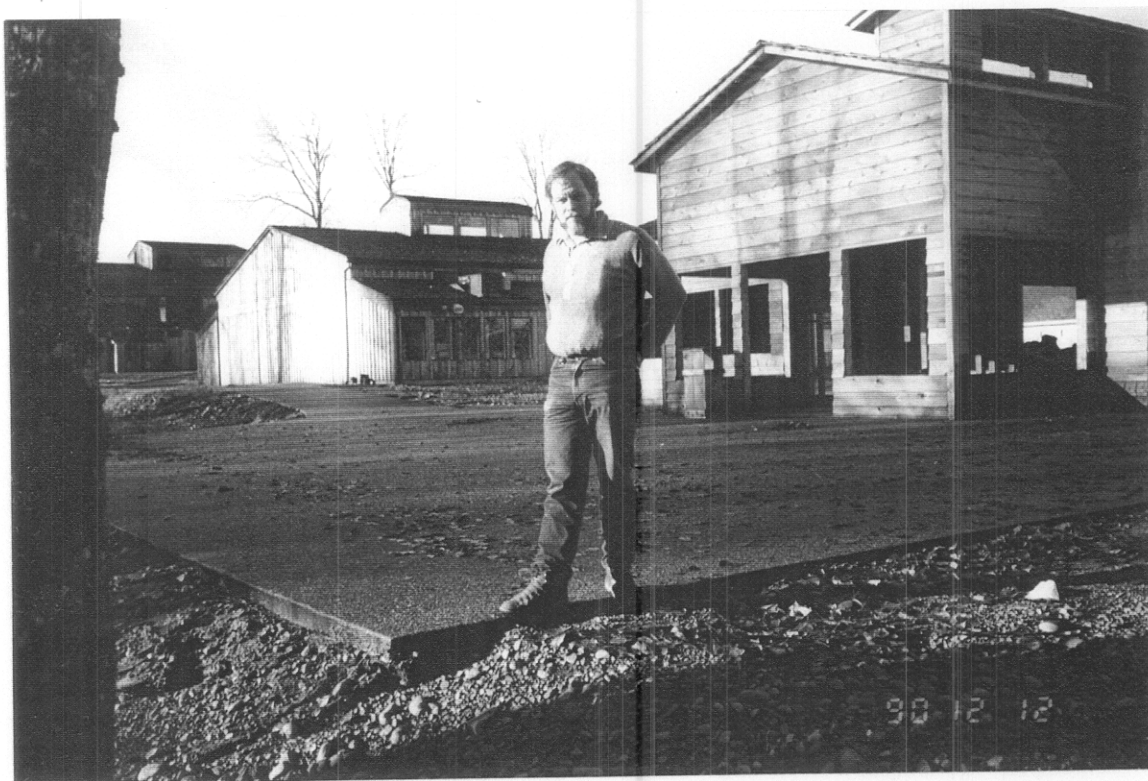
Photo 13 Rear of Native Heritage Centre on Cowichan Way on the left bank upstream of XS-44. December 4, 1990 high water mark indicated by toe of right boot and trash line beyond.
