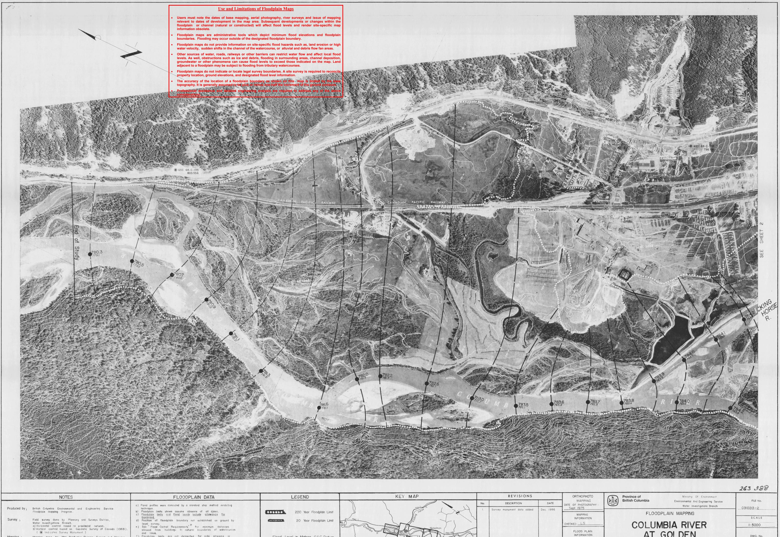
AT GOLDEN DWG. No. f) Floodplain limits are not delineated for side streams or Flood Level in Metres , G.S.C. Datum. Mapping ; Mapping done by Map Production Division, Surveys and Mapping tributaries, except where shown. CHECKED: R.D.Z. a) Contour interval — I metre and greater; Spot elevations shown to 0.1 metres, with accuracy to ± 0.3 metres
