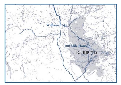
Aquifer 124, located in the 100 Mile House region, is defined by a basaltic bedrock formation. The dashed linear boundaries indicate limit of study area. As data are acquired, the boundary will be extended to encompass the complete basaltic formation.
