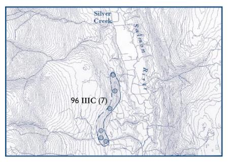
Bedrock aquifer 96, south of Salmon Arm, is defined by the close proximity of a minimum number of wells constructed in the bedrock (area of aquifer development) and the boundary between those wells completed in bedrock and those completed in sand and gravel. The dashed line indicates there was insufficient information to extend the aquifer boundary further upslope. The solid line indicates greater confidence in the boundary based on well and surficial geology information.
