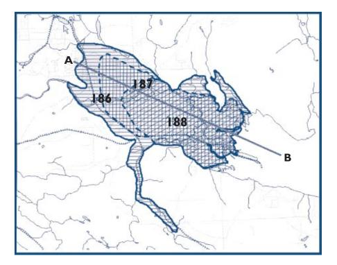
Three aquifers in the Duncan area overlie one another, with less permeable materials separating them. The uppermost aquifer (#186) is a highly vulnerable one that overlies a moderately vulnerable aquifer (# 187), which in turn overlies a low-vulnerability aquifer (#188). The overlapping aquifers are graphically represented in the accompanying cross-section, A - B.
