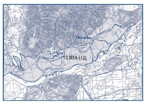
Aquifer 12, a sand and gravel aquifer, is located east of Hatzic Lake on the north side of the Fraser River. It is defined primarily by geologic boundaries and the boundary with a major water body - the Fraser River. The solid line of the boundary indicates a high degree of certainty about the boundary's location.
