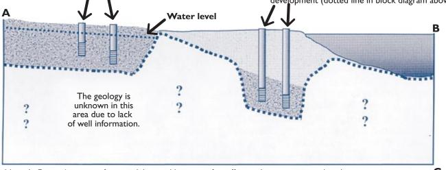
Note: In Figure 6, two aquifers are delineated because of insufficient data to suggeste that there is one continuous **C** aquifer.
