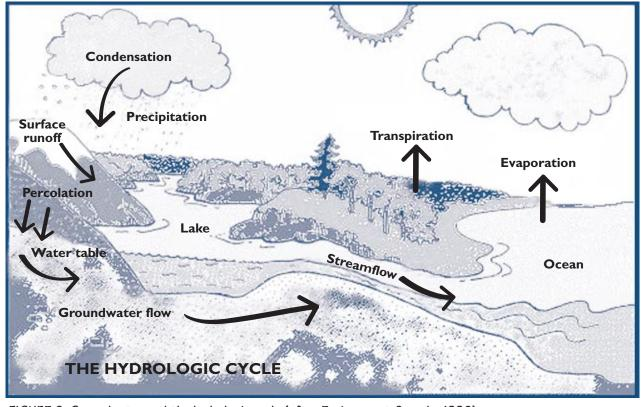
FIGURE 2. Groundwater and the hydrologic cycle (after Environment Canada, 1990)
