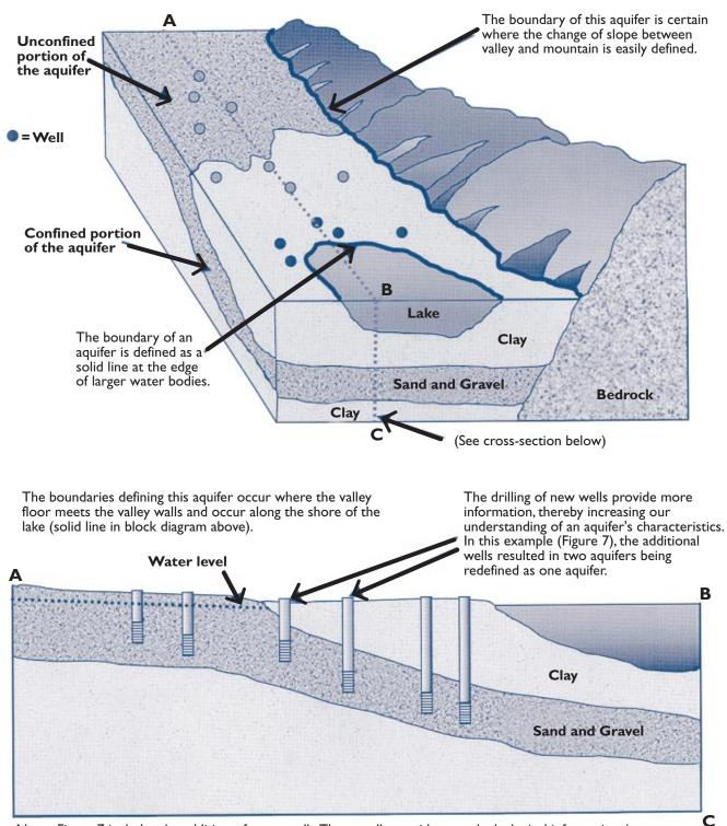
Note: Figure 7 includes the addition of more wells. These wells provide more hydrological information (e.g., lithology information from well logs). This additional information would result in two aquifers becoming one aquifer and its classification would be adjusted accordingly.
