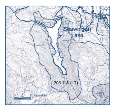
Aquifer 203, a bedrock aquifer located between Duncan and Victoria, is defined primarily by Shawnigan Lake's drainage basin. The dashed line of the boundary indicates a low degree of certainty about the boundary's location.
