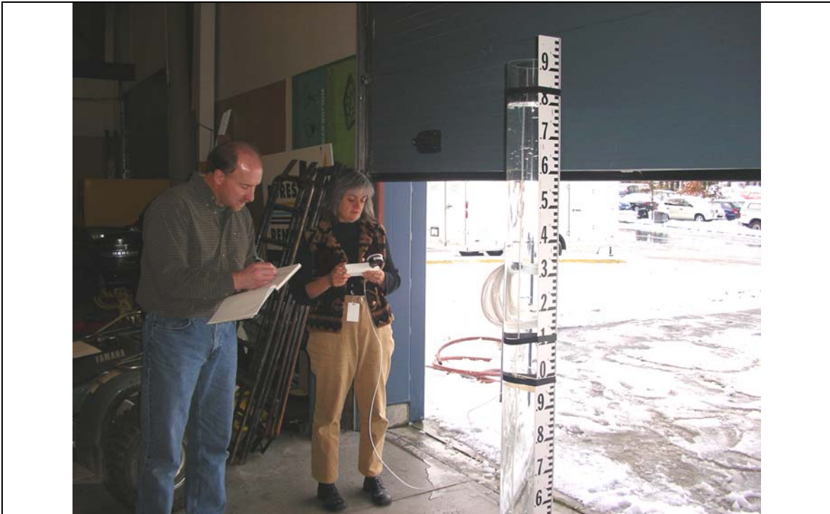
Photo 1. Ministry of Environment staff Pat Lapcevic and Brian Epps testing a submerged air-line water level monitor using a demonstration well.
